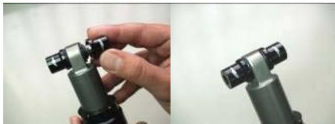
**7.** Insert the screw or supporting axle attached to the shock and compress the suspension at the same time as you firmly tighten the screw. **Stop when you reach 8 Nm for M6 screws or 12 Nm for M8 screws ( 6 and 10 Nm with aluminum screws).**
