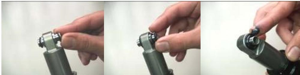
**6.** Next attach the aluminum spacers, having previously compressed them by hand so that they compress the o-rings and fit on the inner ring. While compressing, proceed to reposition the shock into the bicycle.
