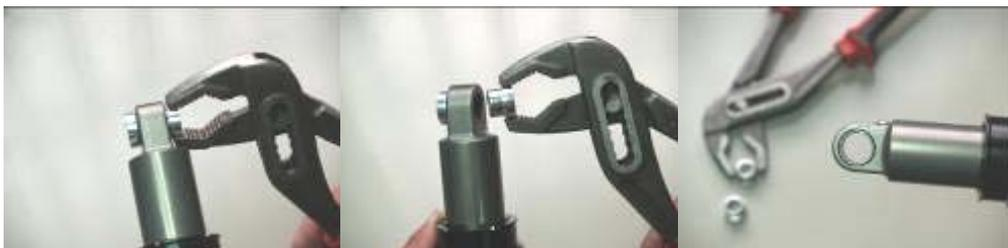
2. Thoroughly grease all pieces of the extractor and insert it in the DU bushing. Check to see that it is properly aligned in relation to the shock eye and then press firmly until the entire assembly comes out the other side. Clean the shock eye and check to make sure it doesn't have any deformations that could impede the installation of the Roller Kit.
