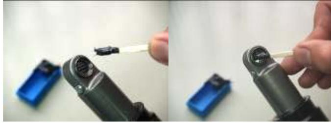
**5.** Position the inner ring (already lubricated) and place the O-rings on top as shown in the photos. Next completely coat both sides of the assembly with grease.
